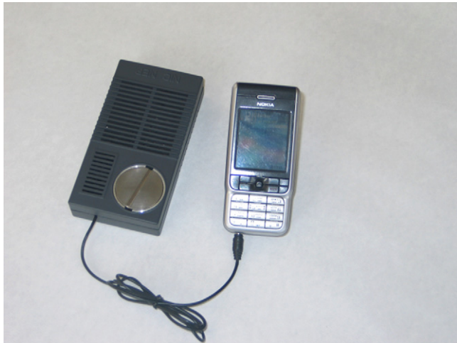
Fig. 1. 2 W PS for cellular phone accumulators charging.
